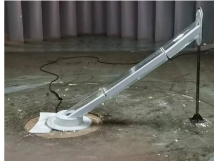
Figure 3. Photo of the inclined Model 0 installed in the test section
